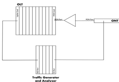
Figure 8. IGMP Group Multicast Testing Configuration
