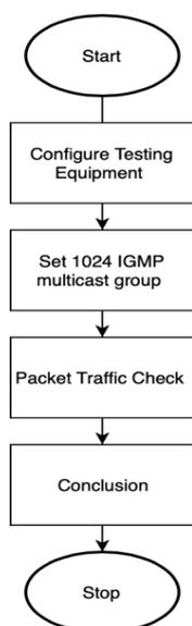
Figure 9. IGMP Group Multicast Testing Flowchart
