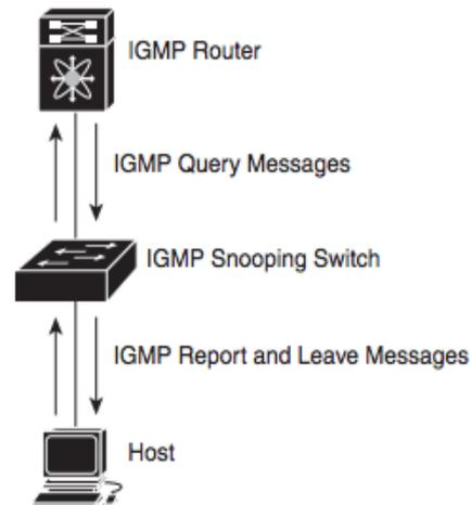
**Figure 13.** IGMP Snooping Source: (Cisco, 2017)
