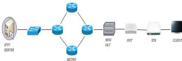
**Figure 5.** IGMP, IGMP Proxy, and IGMP Snooping Testing Configuration
