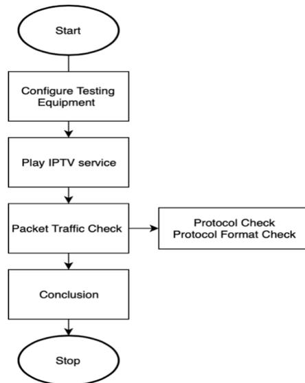
**Figure 6.** IGMP Version Testing Flowchart
