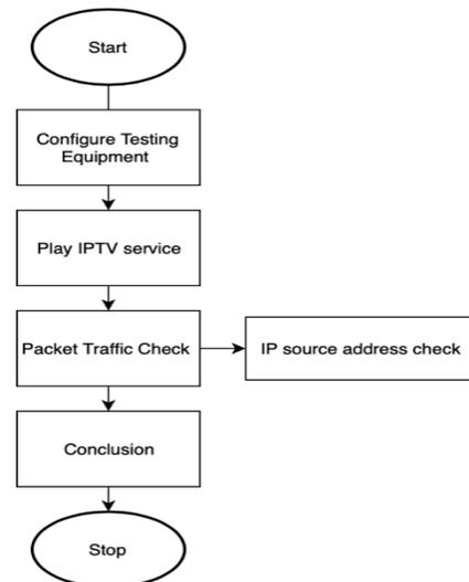
**Figure 7.** IGMP Snooping and Proxy Testing Flowchart
